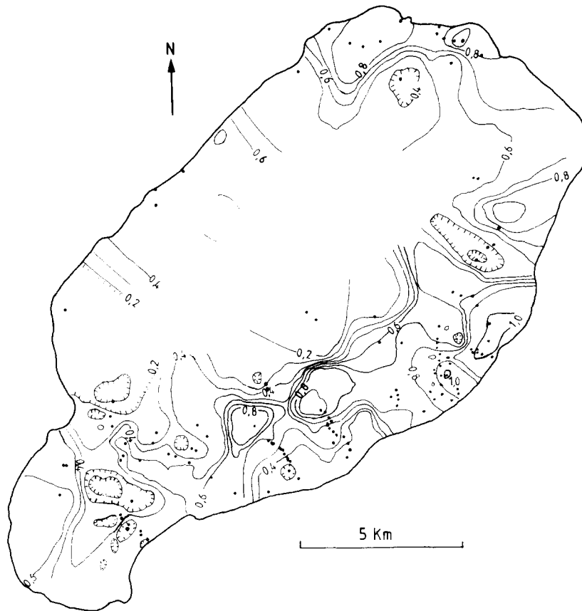
Fig. 10. Contour map of the mean logarithmic xenolith axial ratios over the Criffel pluton. Contours have been machine drawn at the University of St Andrews using an interpolation method based on inverse distance weighting on the four nearest points (Sampson 1975). Measurement sites are indicated by small filled circles.
